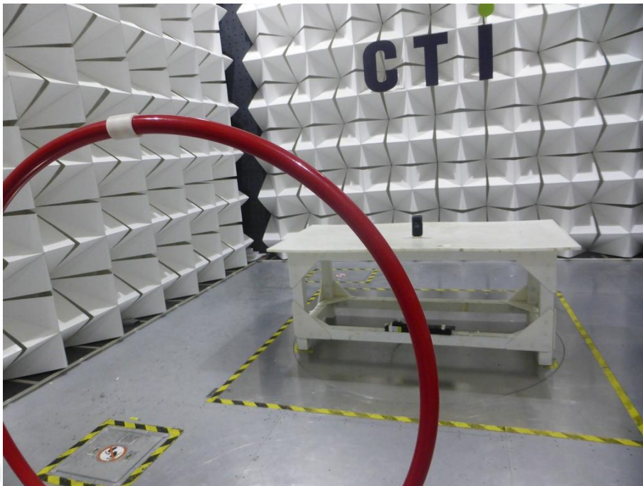
Radiated emission Test Setup (9kHz~30MHz)
