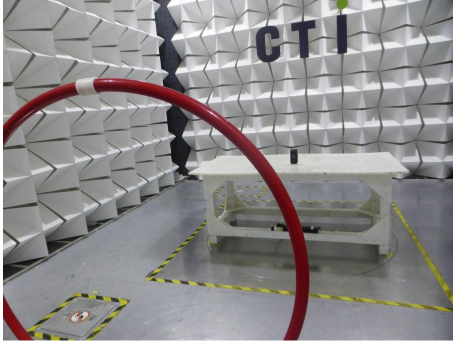
Radiated spurious emission Test Setup-1(9kHz-30MHz)
