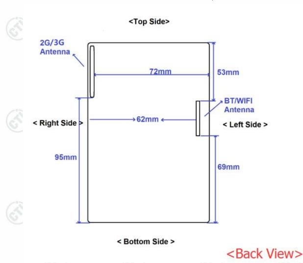
The SAR measurement positions of each side are as below:
