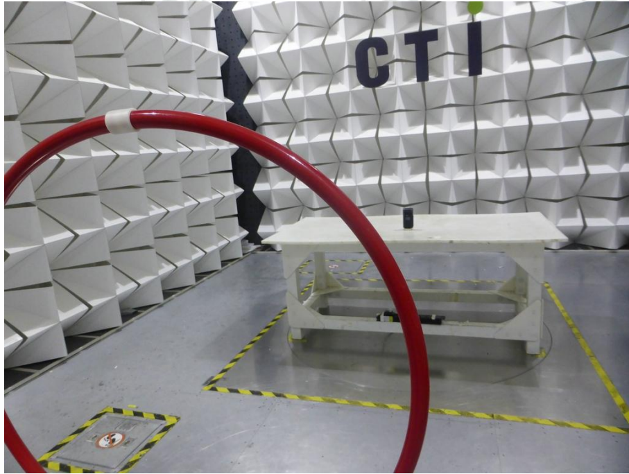
Radiated spurious emission Test Setup-1(9kHz-30MHz)
