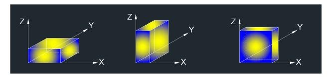
Note: For all radiated test, EUT in each of three orthogonal axis emissions had been tested, but only the worst case (Y axis) data recorded in the report.
