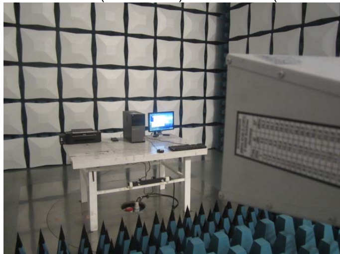
Radiated Emission (above 1GHz) Connect to PC(Down loading)
