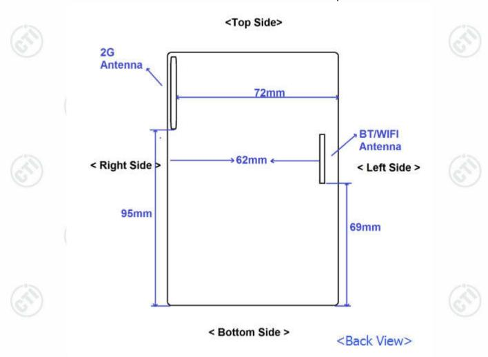
The SAR measurement positions of each side are as below:
