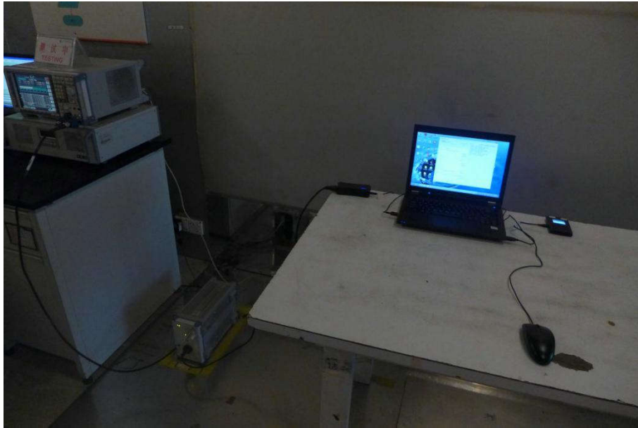
Conducted Emissions Test Setup
