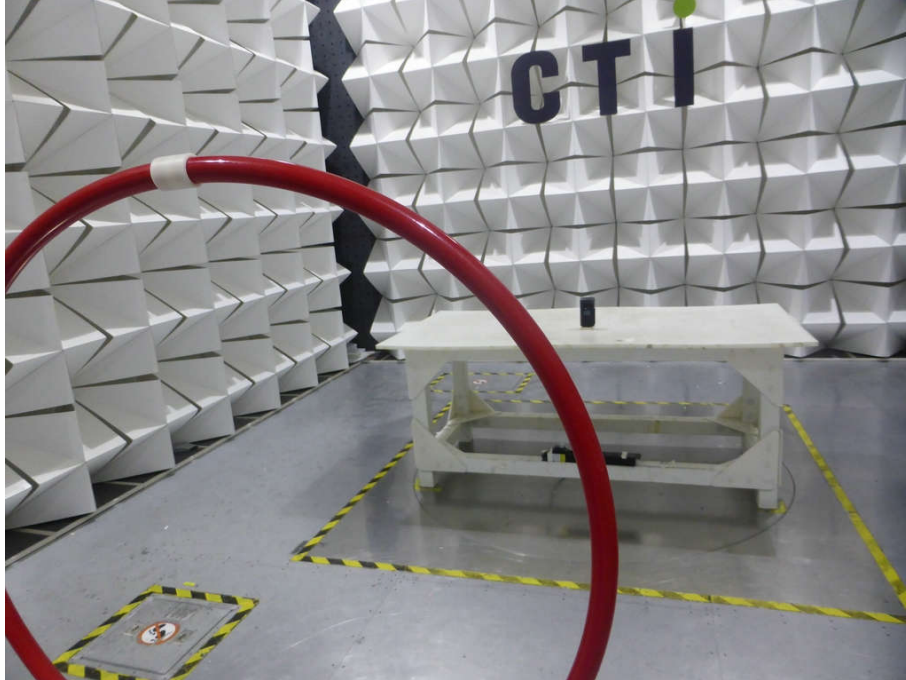
Radiated spurious emission Test Setup-1(Below 30MHz)
