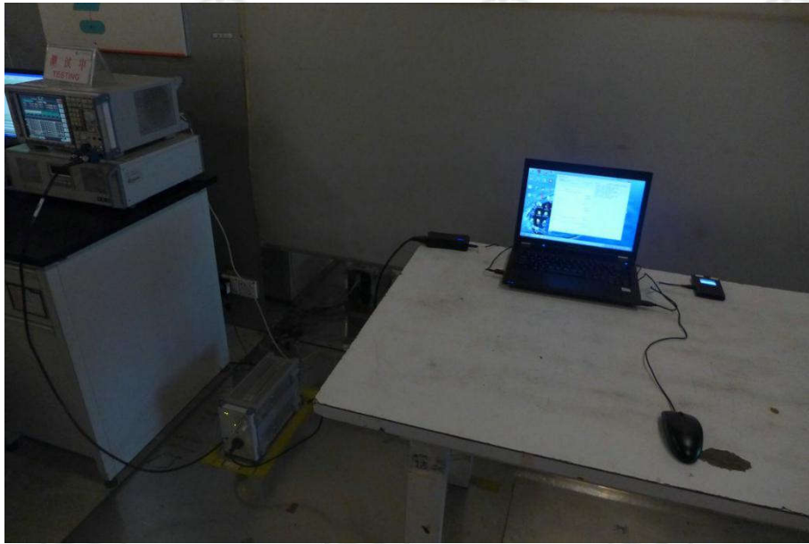
Conducted Emissions Test Setup
