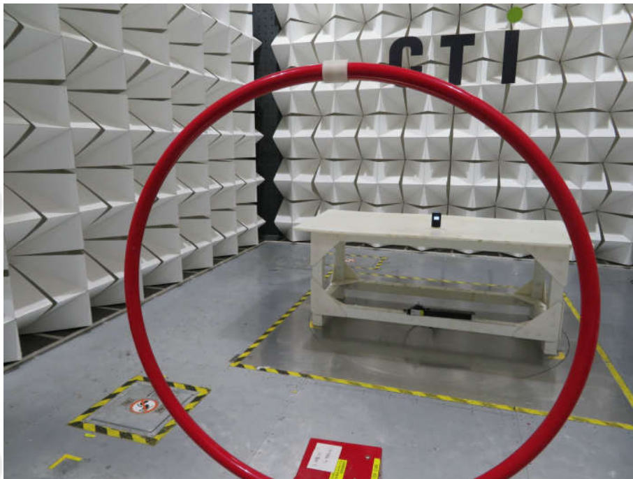
Radiated emission Test Setup (9kHz~30MHz)
