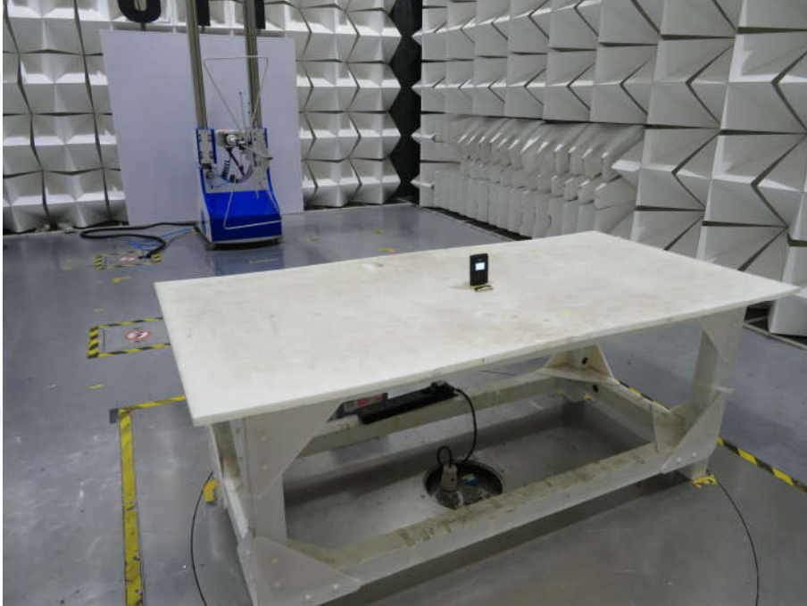
Radiated emission Test Setup (30MHz~1000MHz)
