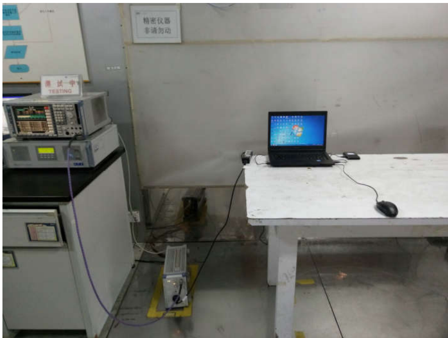
Conducted Emissions Test Setup
