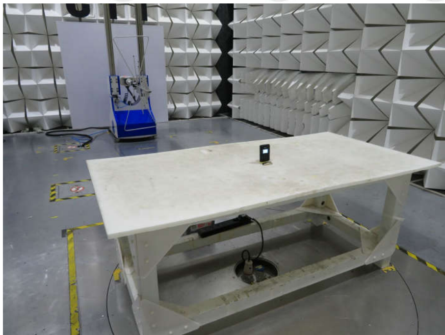
Radiated spurious emission Test Setup-2(30MHz-1GHz)
