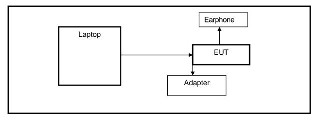
Note: Adapter only use for AC POWER LINE CONDUCTED EMISSIONS testing.
