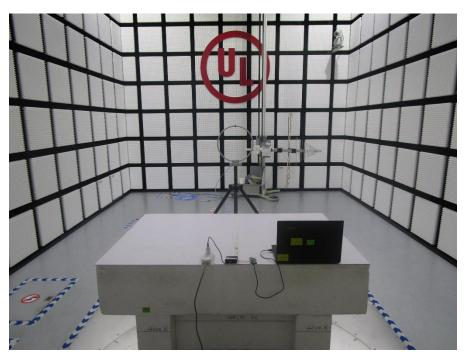
POWERLINE CONDUCTED EMISSIONS MEASUREMENT SETUP
