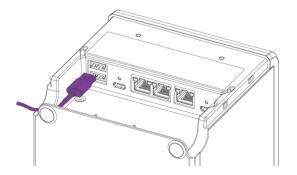
2. Plug in the remaining Micro-USB side into the bottom of the puck.
