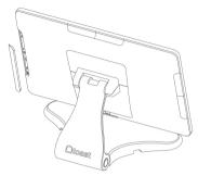
Plug in the end of the Micro-USB cable paired with the cover and screws. Then screw in the plate to the terminal.
