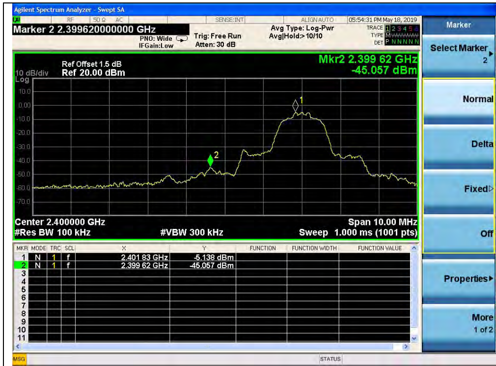
(Channel = 0, Band edge, \pi/4 -DQPSK)
