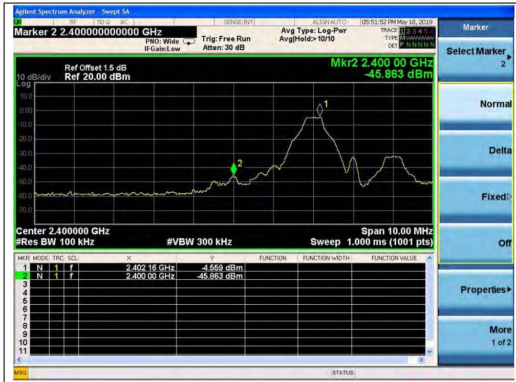
(Channel = 0, Band edge, GFSK Mode)
