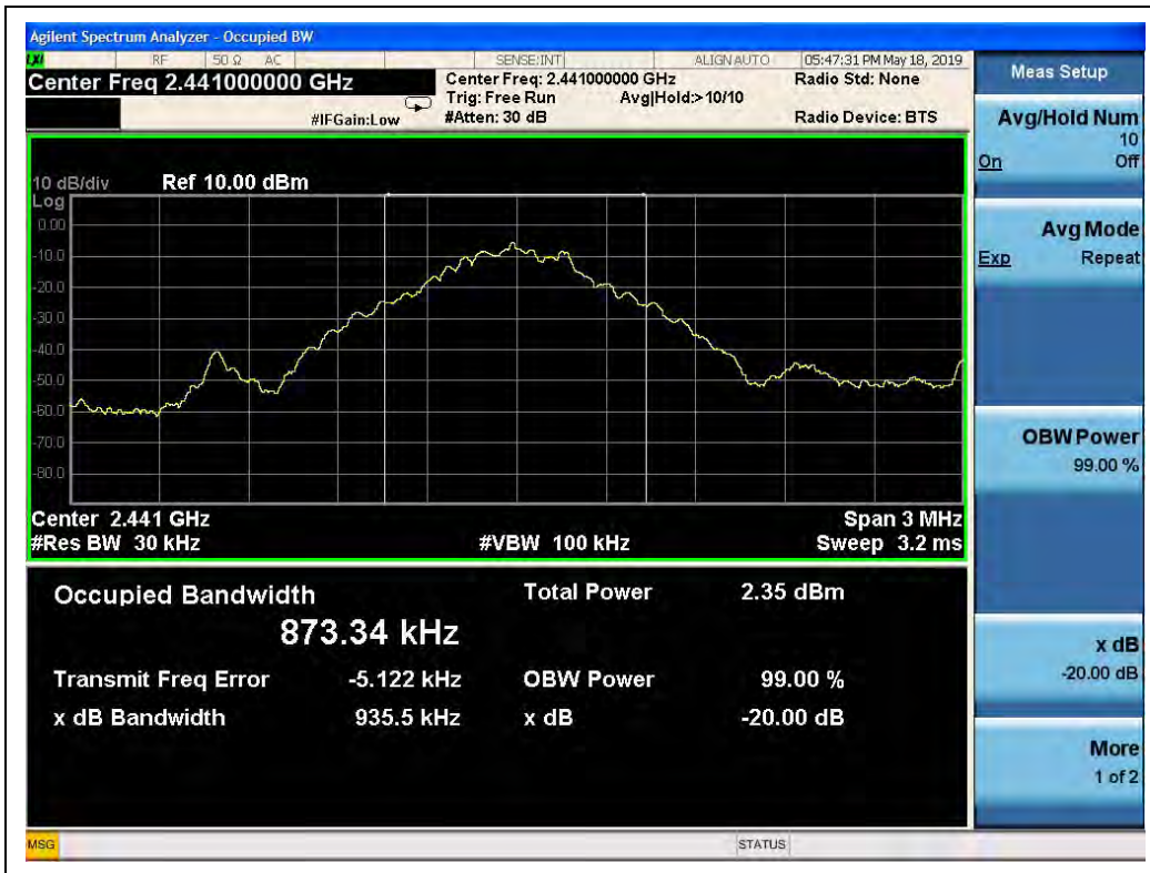
(GFSK, Channel 39, 2441MHz)
