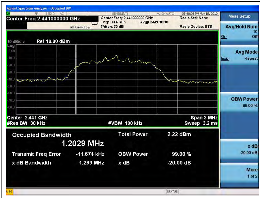
( \pi/4 -DQPSK, Channel 39, 2441MHz)
