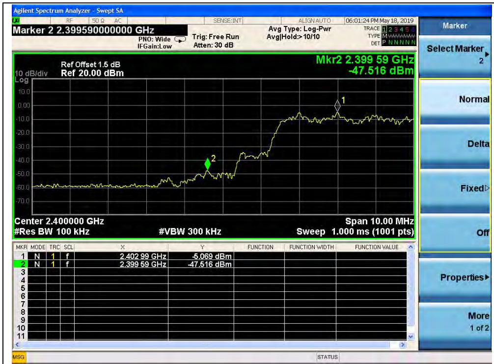
(Channel = 0, Band edge with hopping on, 8-DPSK)
