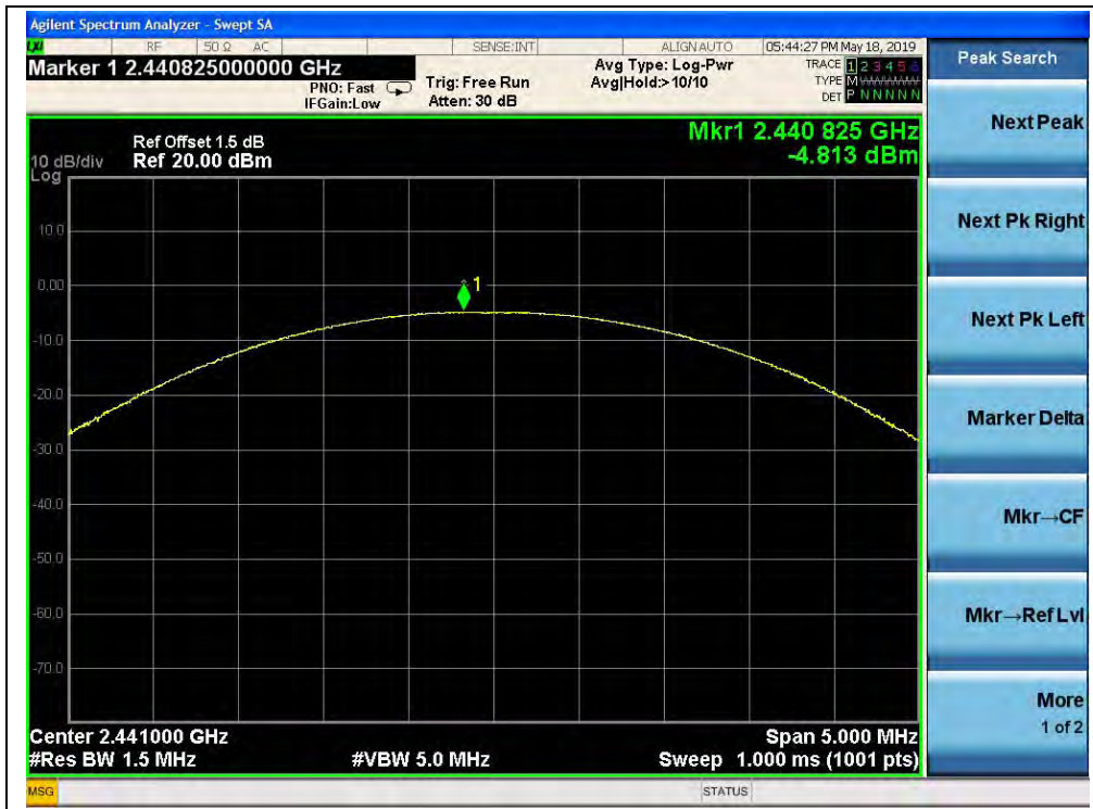
( \pi/4 -DQPSK, Channel 39, 2441MHz)
