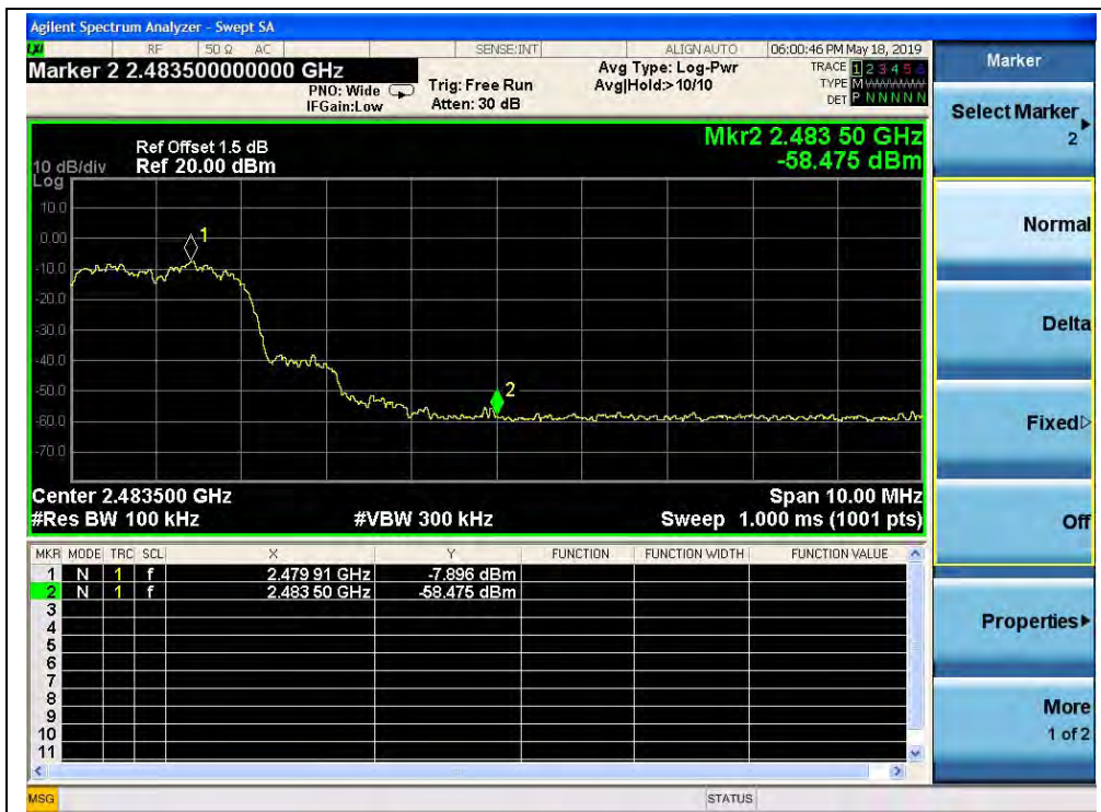
(Channel = 78, Band edge with hopping on, 8-DPSK)
