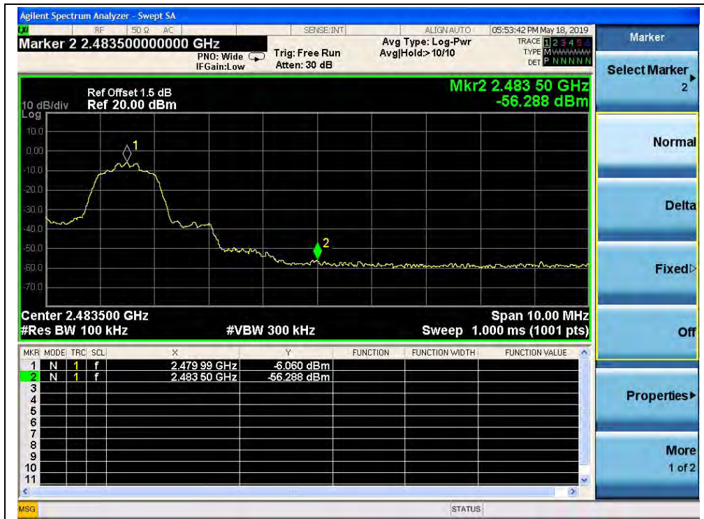
(Channel = 78, Band edge, \pi/4 -DQPSK)
