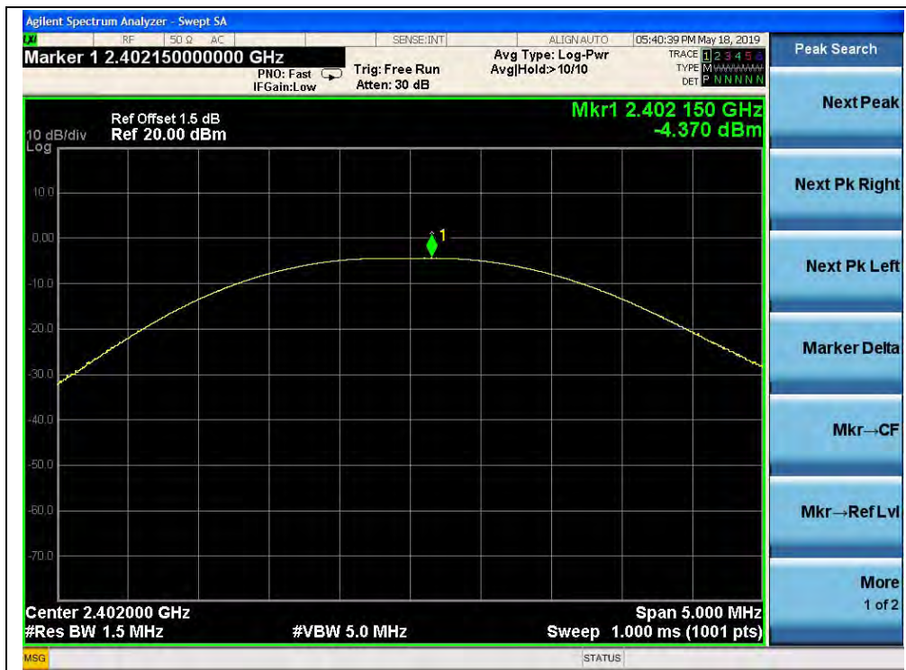
(GFSK, Channel 0, 2402MHz)
