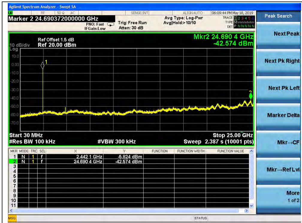
(Channel = 39, 30MHz to 25GHz, GFSK Mode)
