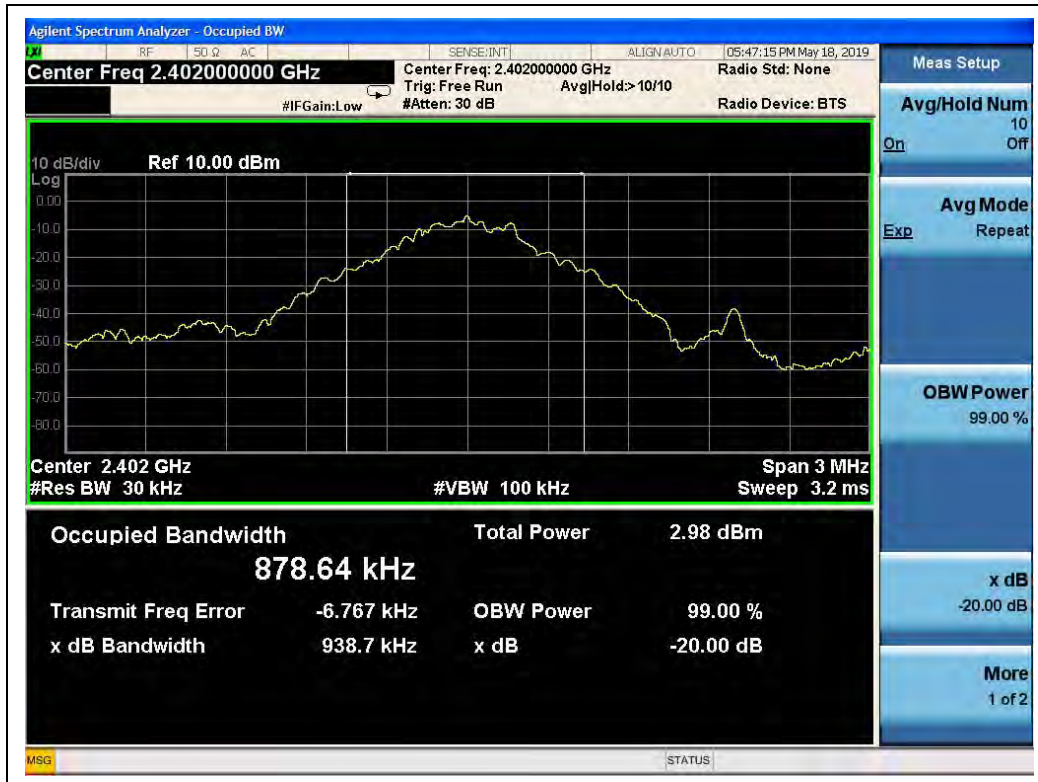
(GFSK, Channel 0, 2402MHz)
