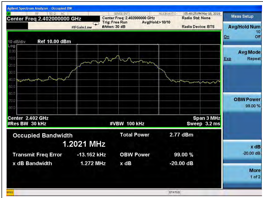
( \pi/4 -DQPSK, Channel 0, 2402MHz)
