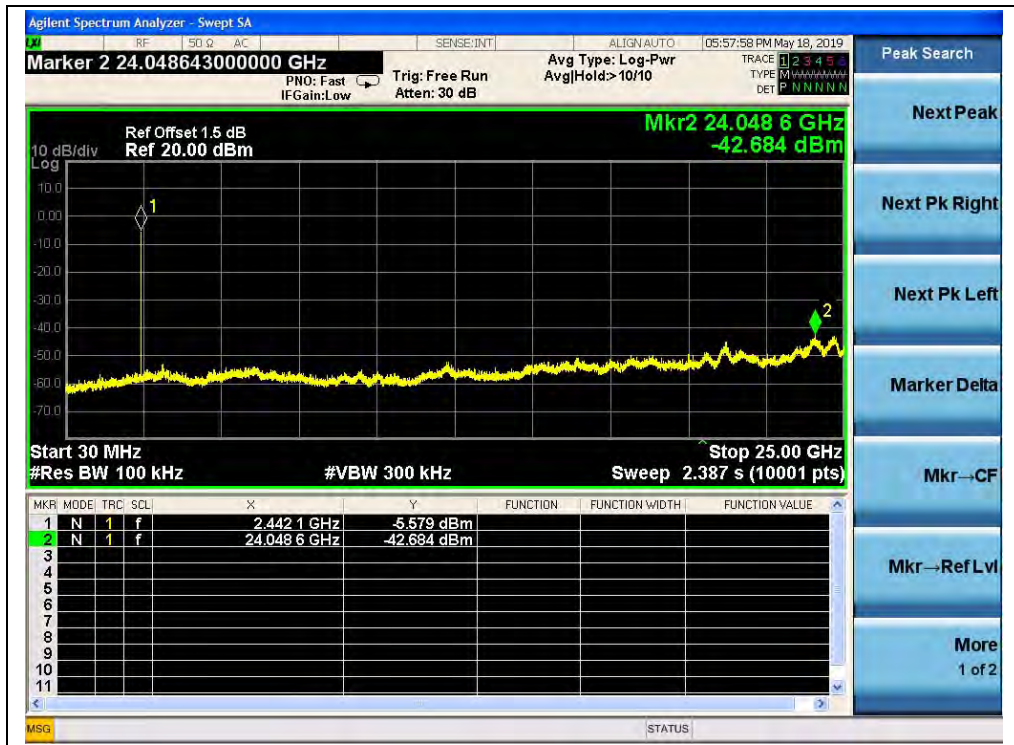
(Channel = 39, 30MHz to 25GHz, \pi/4 -DQPSK)
