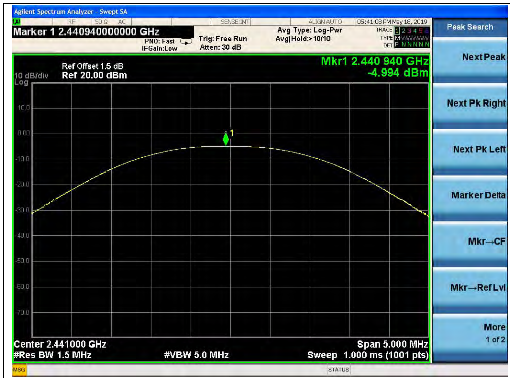
(GFSK, Channel 39, 2441MHz)
