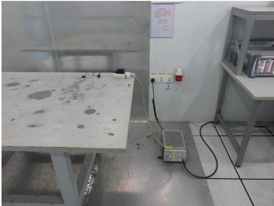
1 Photo of Conducted Emission Test
