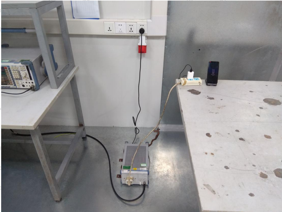
Photo of Conducted Emission Measurement
