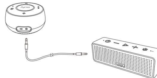
You can connect Eufy Genie to an external speaker with the supplied AUX cable (5 ft).
