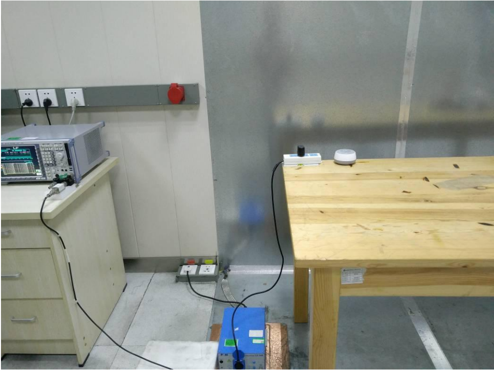
FCC RADIATED EMISSION TEST SETUP BELOW 1GHZ
