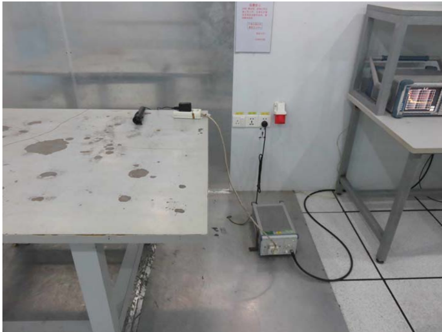
1 Photo of Power Line Conducted Emission Measurement
