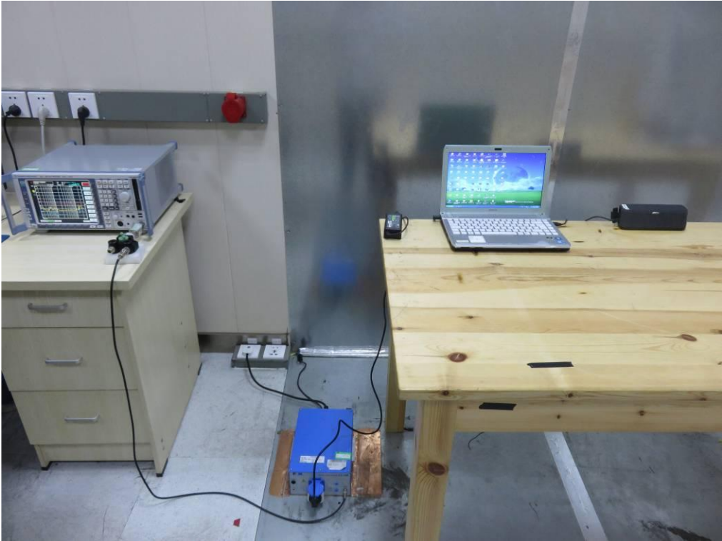
FCC RADIATED EMISSION TEST SETUP
