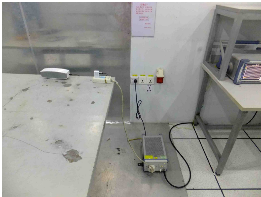
1 Photo of Conducted Emission Test
