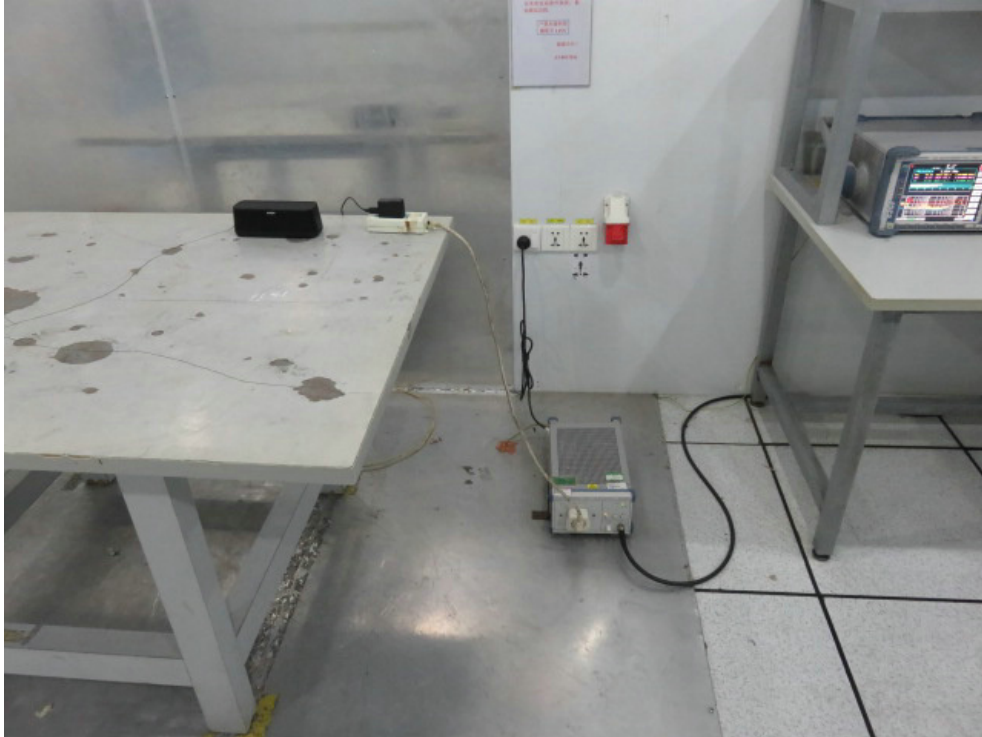
Photo of Conducted Emission Measurement
