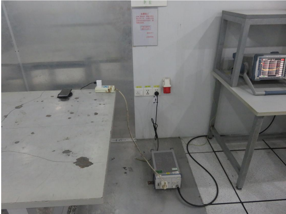
Photo of Conducted Emission Measurement
