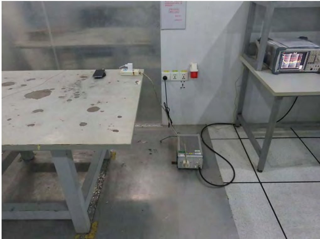
1 Photo of Conducted Emission Test
