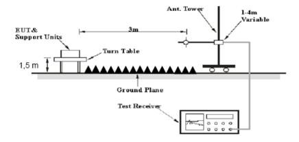
The radiated emission and out of band emission tests were performed in the 3 meters chamber test site, using the setup accordance with the ANSI C63.10-2013 The specification used was the FCC 15.209/15.205 and FCC 15.249 limits.
