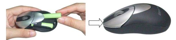
3. After the AAA Batteries have been installed into your Mouse properly, the sensor LED inside your Mouse will light up.
