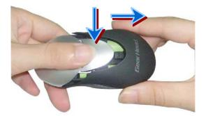
2. Install two AAA Batteries into your Mouse following the battery orientation guide in the battery bay and then replace the Battery Compartment Cover back onto your Mouse until it securely locks.
