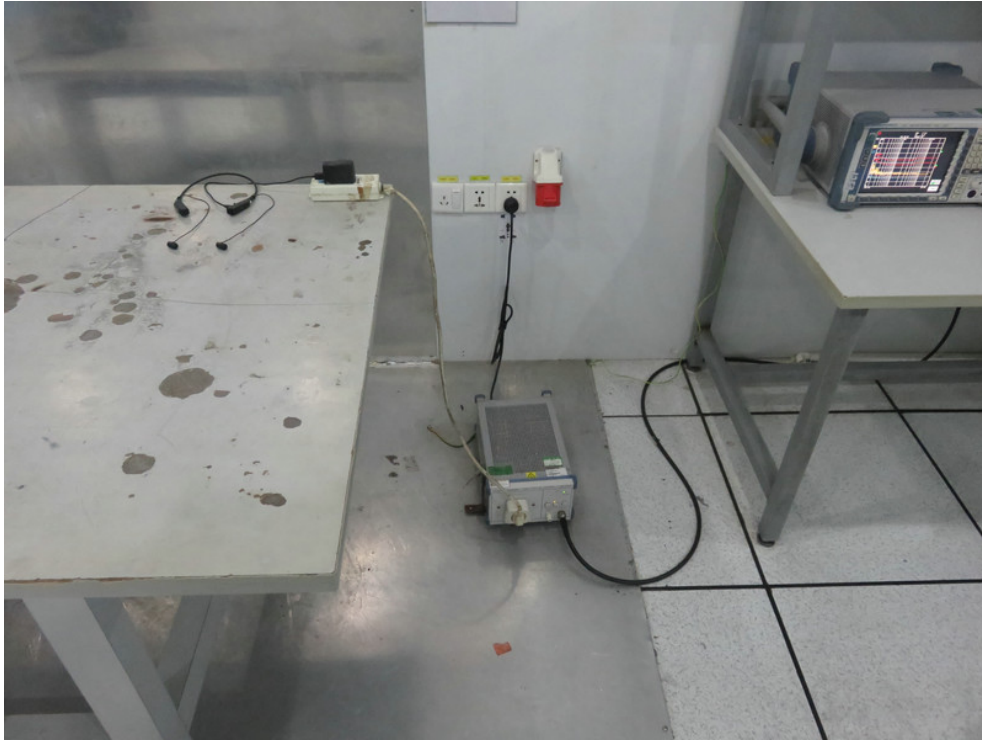
Photo of Radiation Emission Test
