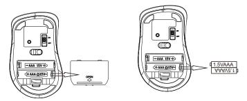
3.Turn the power switch to "on", press and hold the 'connect button' on the bottom of the mouse for three seconds, you will now see the scroll wheel flashing blue. The mouse is now in pairing mode.
