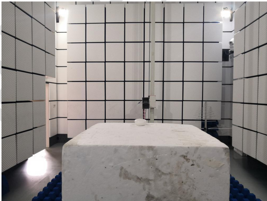
Radiated spurious emission Test Setup-3(Above 1GHz)
