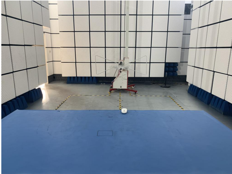
Radiated emission Test Setup-2 (30MHz~1GHz)
