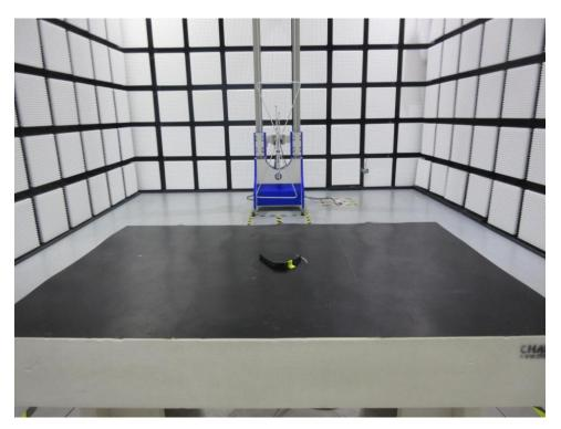
Radiated Emission test Above 1GHz
