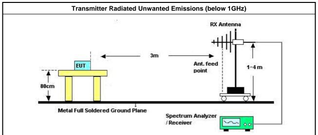
Electric field tests shall be performed in the frequency range of 30 MHz to 1000 MHz using a calibrated bi-log antenna.
