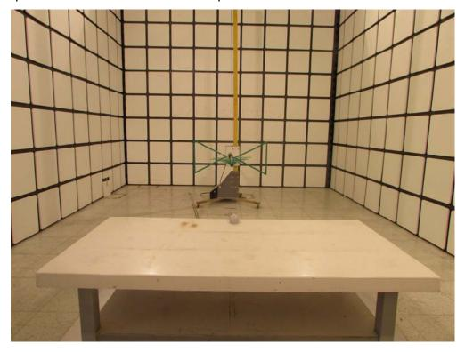
Description: Radiated Emission Test Setup for 1~18GHz
