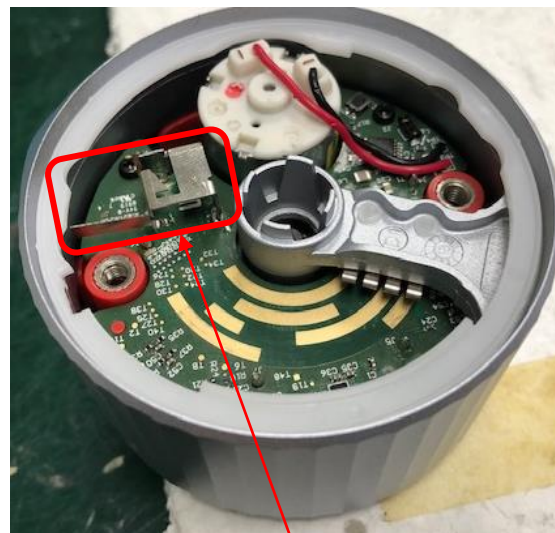
Dual Band Antenna Antenna height (max) : 7.0mm
