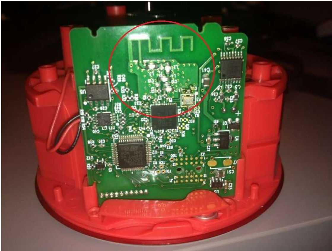
ASL-01 RF Section copied from Texas Instruments Keyfob reference design
