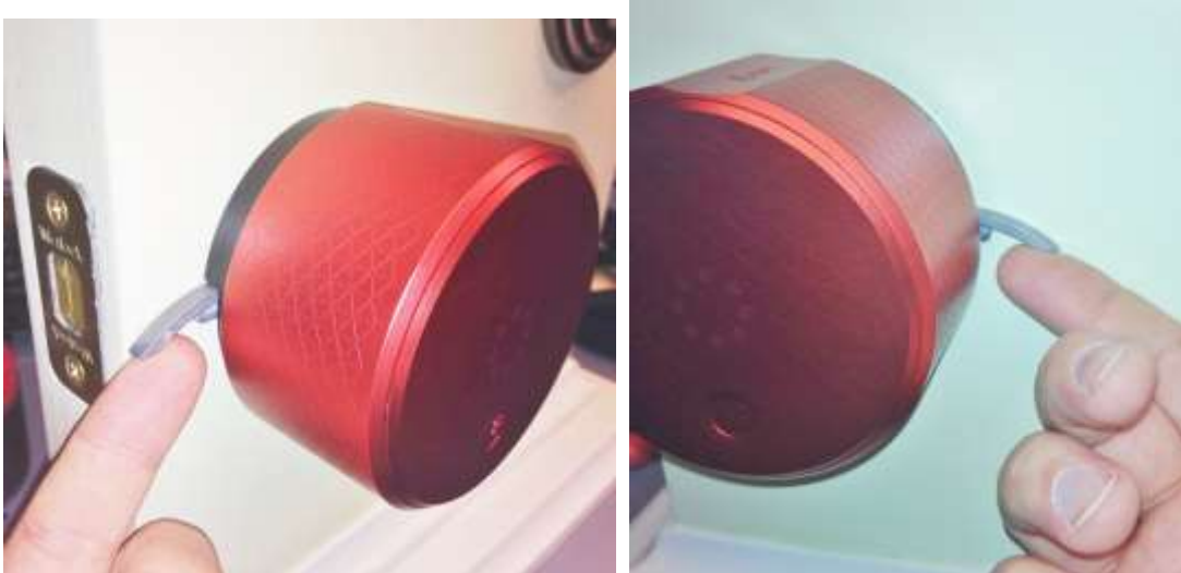
Lift the mounting tabs on both sides of the lock until they are in the open position.
