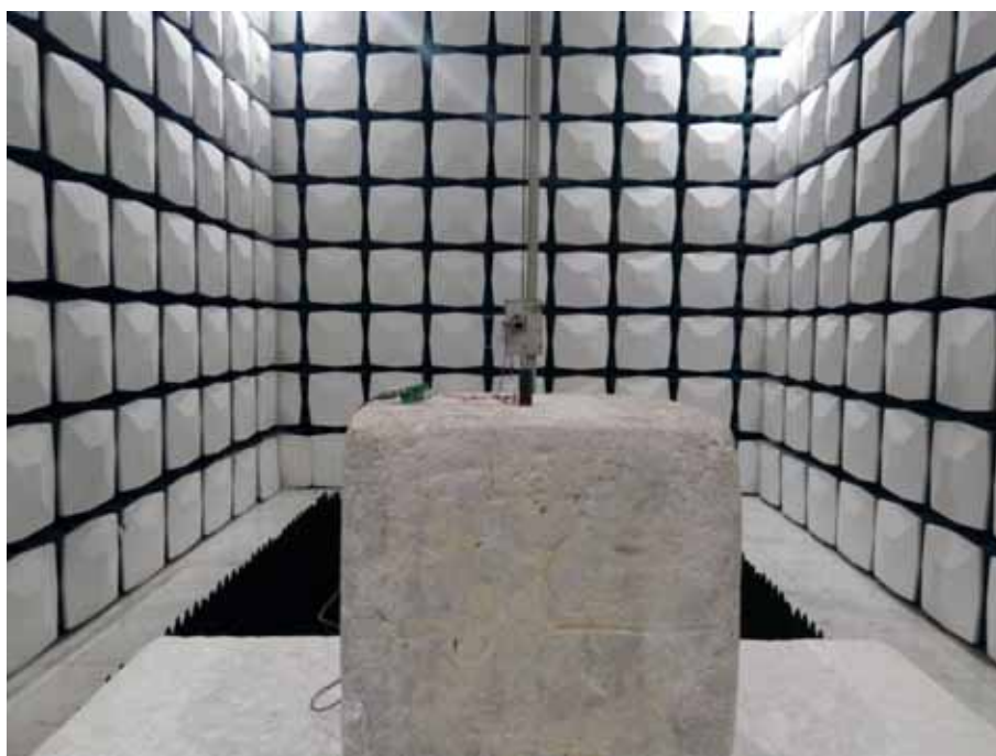
Description: Radiated Emission Test Setup for 18~25GHz
