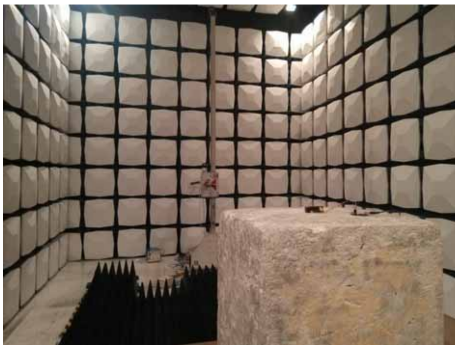
Description: Radiated Emission Test Setup for 18~25GHz
