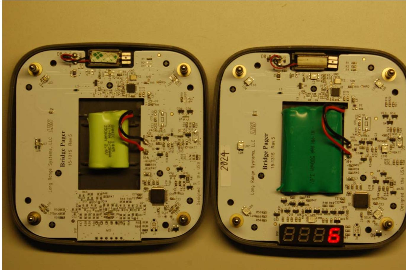
The back side of the PCBA is shown below. The only difference to note is that the RX-CS6 does not have an LED and a Phototransistor populated in the upper, right corner. These parts support light communication between stacked RX-CS7s.
