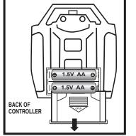
**EACH CONTROLLER USES 2 X 1.5 "AA" SIZE BATTERY** (NOT INCLUDED)
