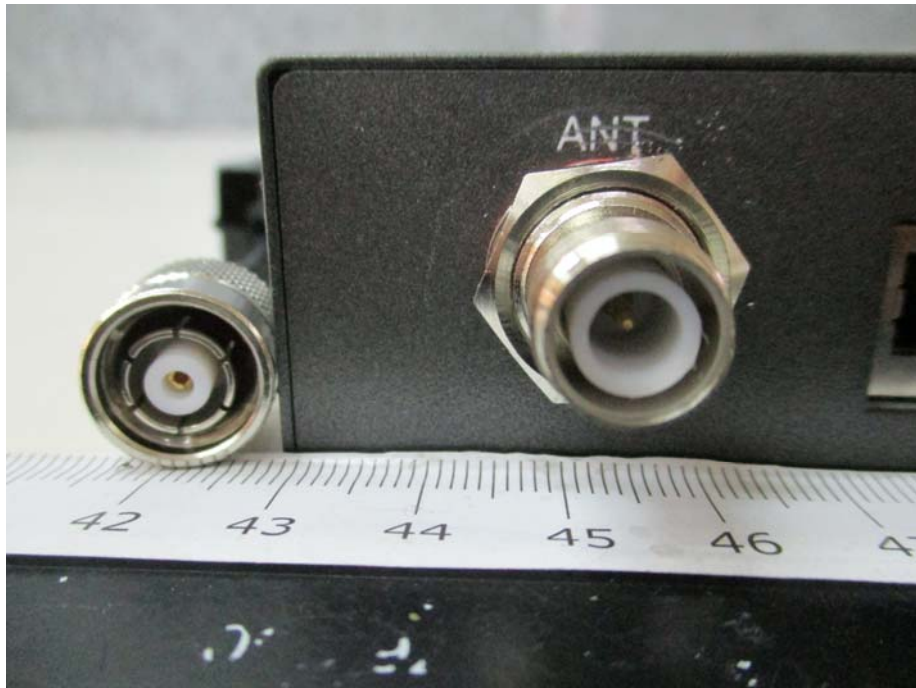
Rear closer view of the antenna port & connector of the antenna
