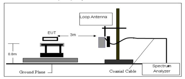
(B) Radiated Emission Test-Up Frequency 30MHz~1GHz
