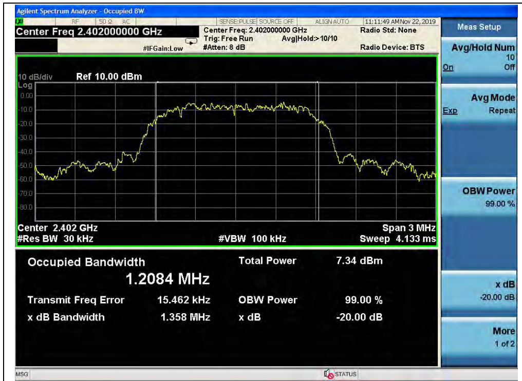
( \pi/4 -DQPSK, Channel 0, 2402MHz)
