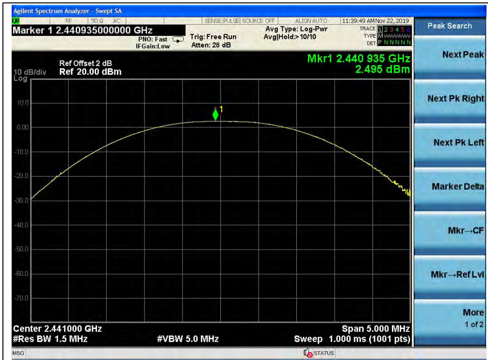
(GFSK, Channel 39, 2441MHz)
