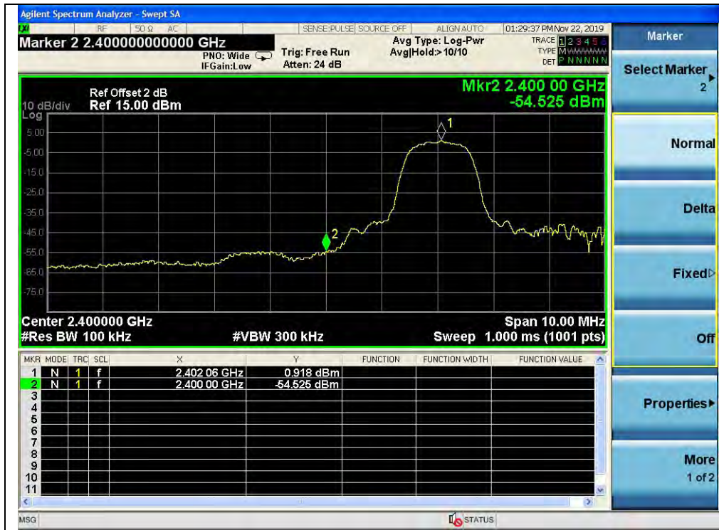
(Channel = 0, Band edge, \pi/4 -DQPSK)
