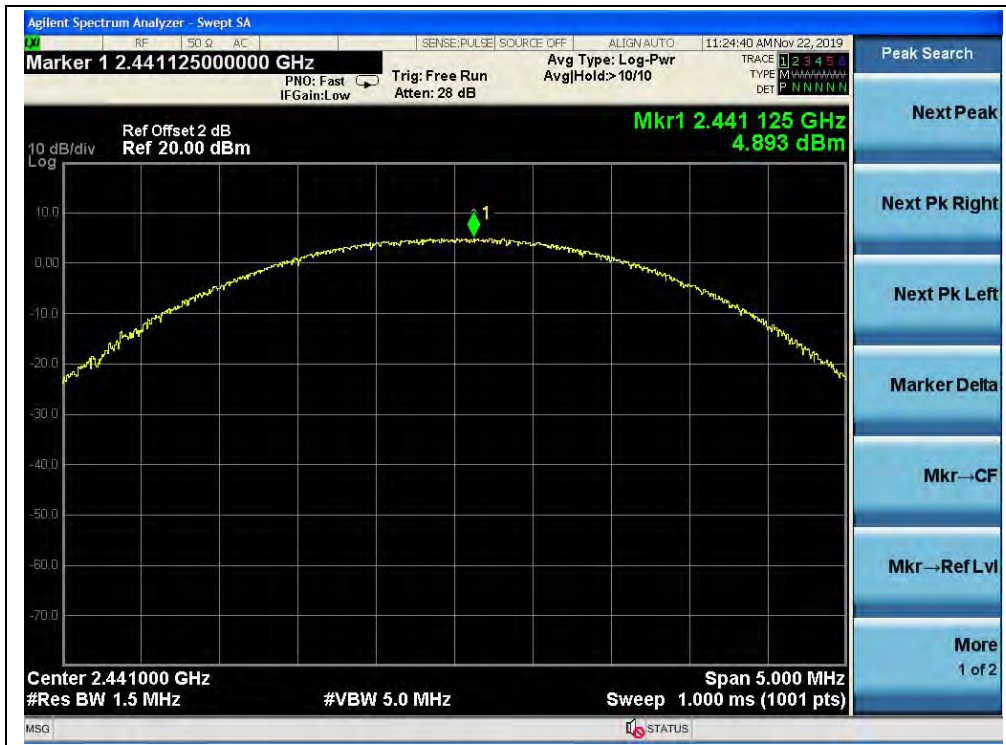
( \pi/4 -DQPSK, Channel 39, 2441MHz)
