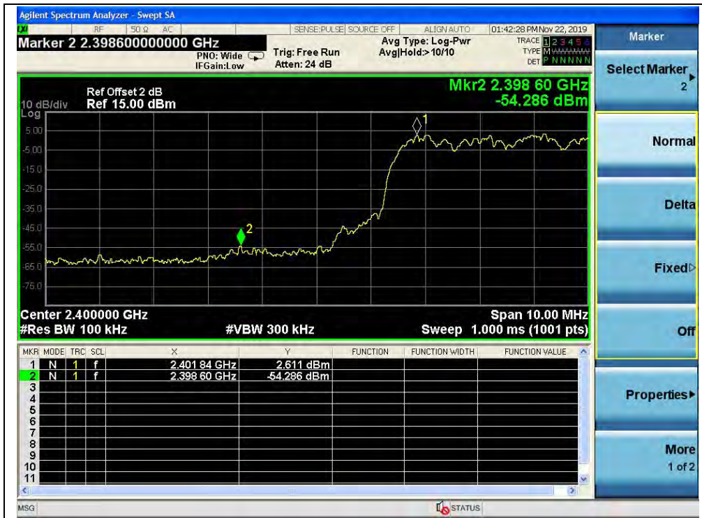
(Channel = 0, Band edge with hopping on, 8-DPSK)
