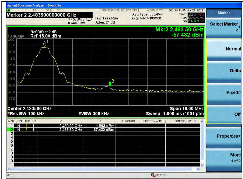
(Channel = 78, Band edge, GFSK Mode)
