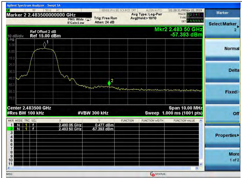
(Channel = 78, Band edge, \pi/4 -DQPSK)
