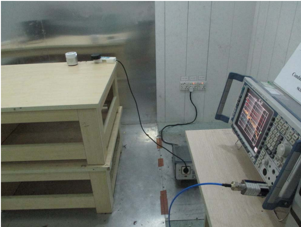
FCC RADIATED EMISSION TEST SETUP
