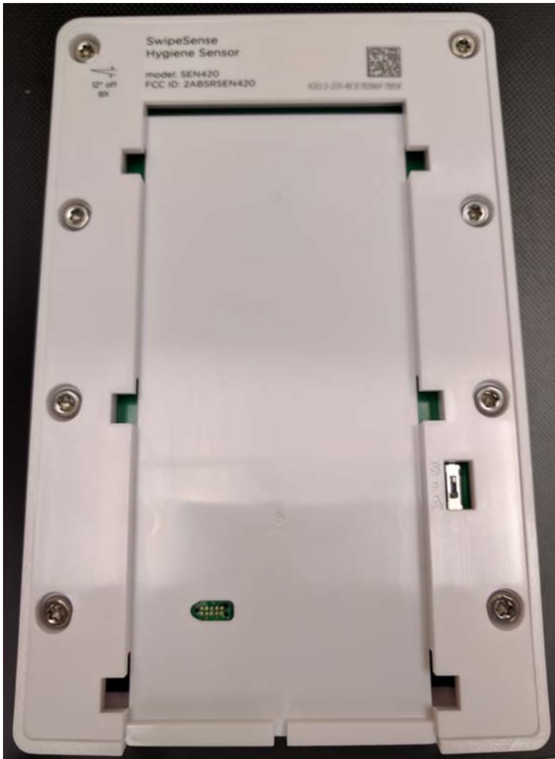
Figure 3 - SwipeSense Hygiene Sensor back view
