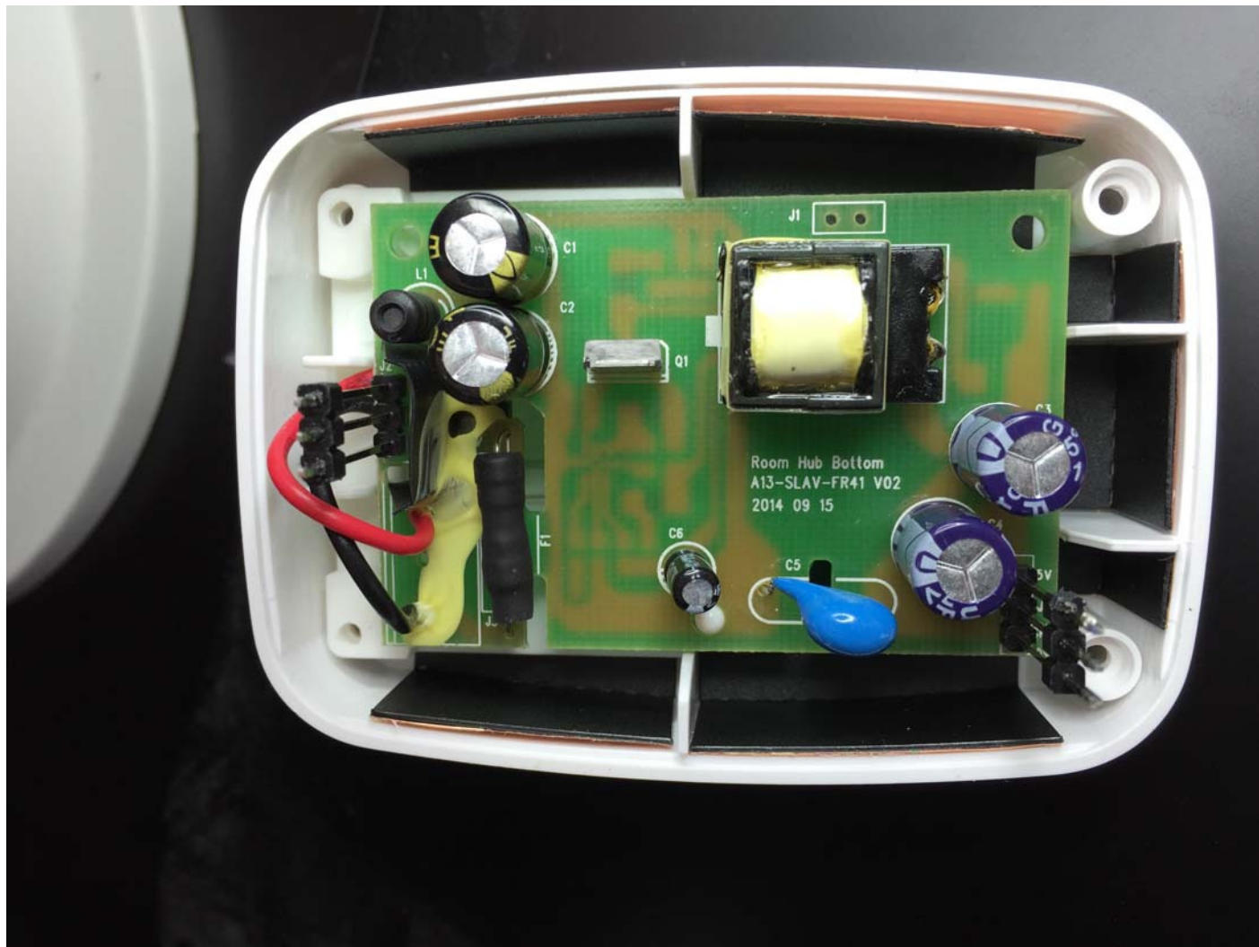
Figure 2 - SwipeSense Location Hub top view of power supply PWB
