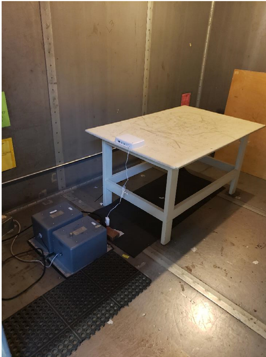
Figure 7. Conducted Power line Emissions Test Setup
