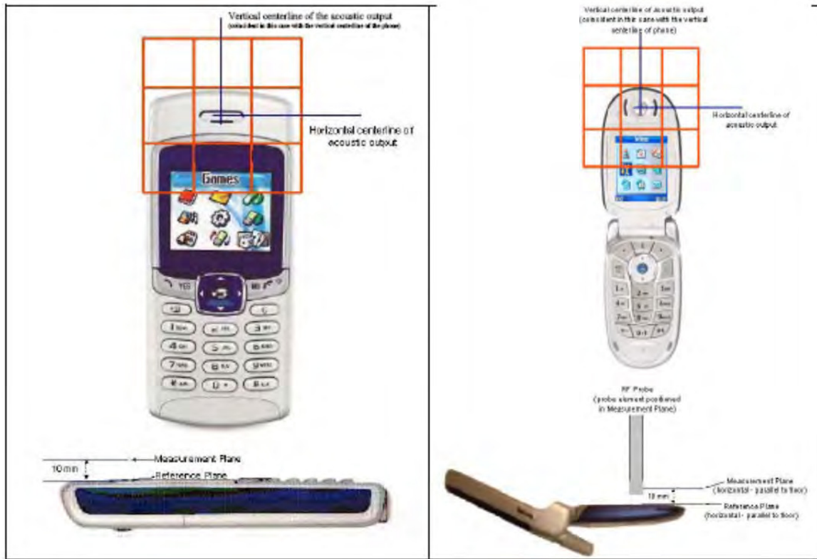
Reference and plane for RF emission measurements
