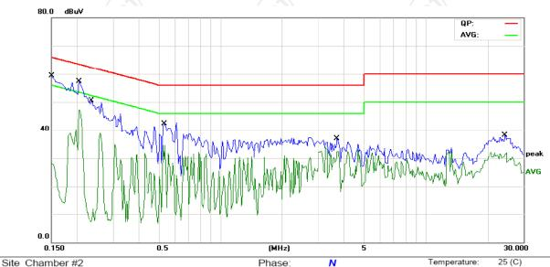
Limit: FCC Part 15B Class B Conduction(QP)
