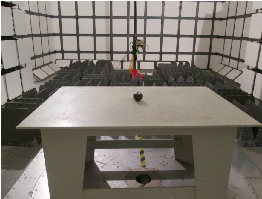
Radiated Emissions View (Above 1 GHz)
